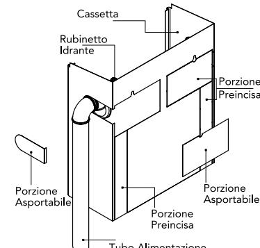
**CASSETTA PER IDRANTI A MURO SERIE TEXAS® "S" CON LASTRA TRASPARENTE INFRANGIBILE RIPORTANTE LE ISTRUZIONI D'USO**
